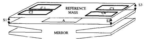
Fig. 5. On the reference mass upper plane (the one above the mirror top) the electrodes are differentiated for creating tilting and stabilizing forces on the mirror. The variable potentials are given to the condensers  $C_1 \dots C_4$ , driven by three sensors  $S_1 \dots S_3$ .
