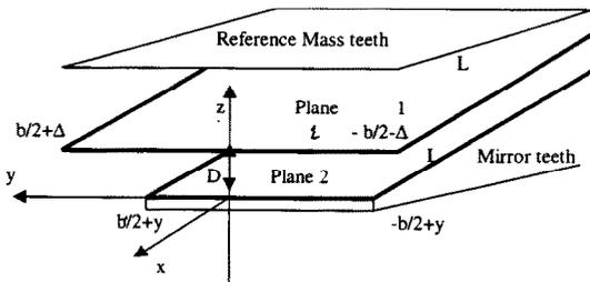
Fig. 6. The reference system used for evaluating the pendulum frequency. The mirror is pendulating along the  $y$  axis.
