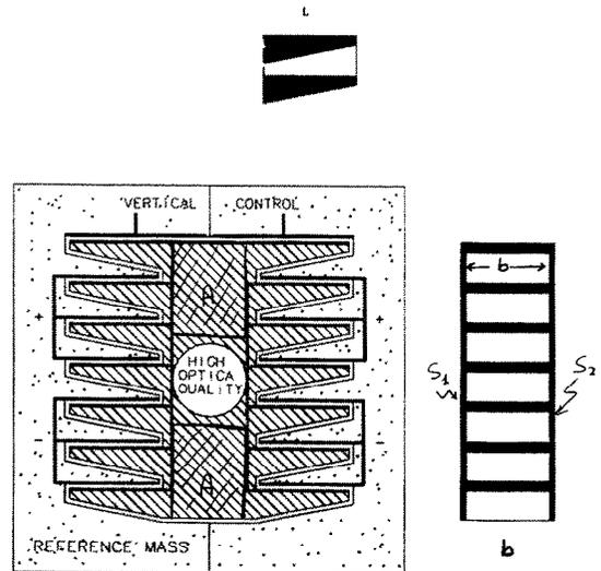
Fig. 3. (a) Mirror and reference mass: both have been carved in two monolithic bulks of optical silica or sapphire. (b) Side view of the mirror: the mirror teeth are all connected by the two optical surfaces,  $S_1, S_2$ , and allow a more rigid structure.
