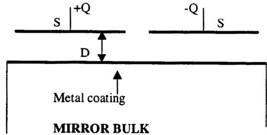
Fig. 2. The topologically deformed configuration originating from the diagram shown in Fig. 1. With this configuration the mirror can be levitated without any wire connection.
