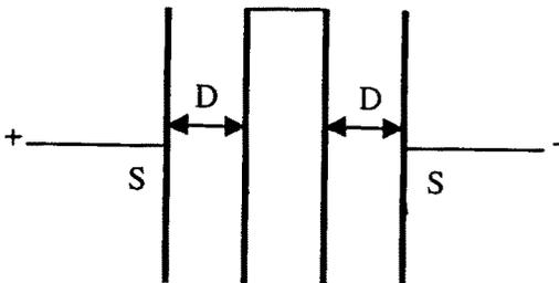
Fig. 1. Two condensers in series; the topological deformation of this diagram can lead to a wireless electrostatic levitation of a test mass.
