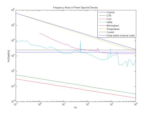
This gives us the level of noise across all frequencies. In order to determine how this translates to linewidth, we need to estimate a bandwidth of the noise (if we were to imagine taking frequencies up to infinity, how far would we see significant noise?). If we take the bandwidth of our noise to be 1 GHz, this translates to a linewidth of
