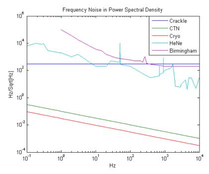
Based on the possible experiments we could perform, we settle on using the Crackle experiment since it has the highest noise requirement and will therefore be the easiest standard to meet.
