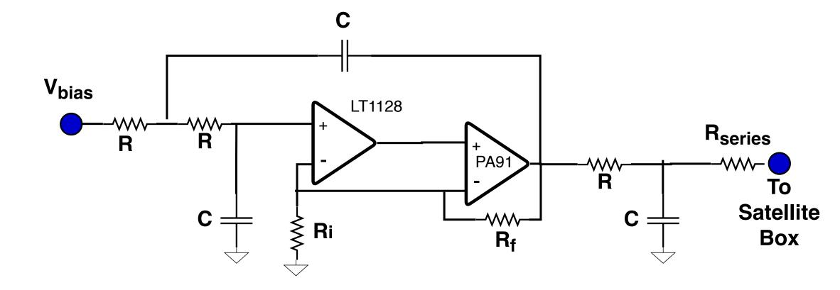
$R_f/R_i$  is used to set a DC gain of x15 so that DAC range of +/-10V is translated to +/- 150V.
